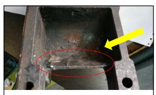
Spring bracket worn out and welded since damaged due to non replacing rubber element on time
