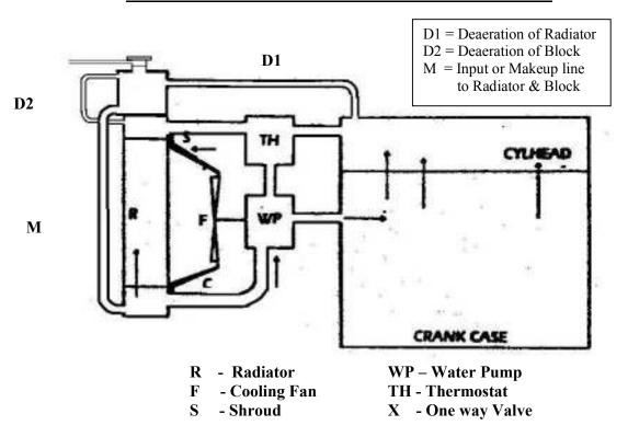
2.2 Use of Ethylene glycol based coolants for better cooling, anti-corrosion and antifreeze properties. The **boiling temperature of this coolant is higher** than ordinary coolant media; hence the **loss of evaporation is greatly reduced** by using these coolants.
