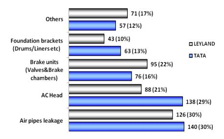
Air leakages and AC Head failures constitute major share in Brake System failure in both Tata & Ashok Leland Area.
