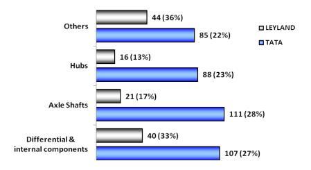
The worn out Half axles shall be replaced during Sch-III/IV maintenance to prevent enroute breakdowns. The splined portion of Wheel Hubs in Tata and studs/stud bores in Ashok Leyland shall be checked thoroughly during Sch-III/IV maintenance.
