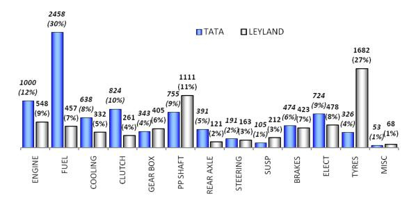
It could be inferred from the critical analysis of breakdowns occurred during the year 2013-14 that the failures on account of very few systems are contributing to the high rate of breakdowns in both Tata and Leyland areas. The following *micro level analysis* of breakdowns in each system helps in identifying the common deficiencies and scope for paying extra attention to the areas where the rate of failures is on high side.
