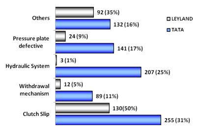
Clutch riding by the Drivers is one of the main causes for such a high rate of clutch related breakdowns in both Tata & Leyland areas. This is more prevalent in Tata area owing to hydraulic clutch actuation fitted on these vehicles. Proper
