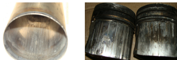
Severe scoring on Cylinder Liner & Pistons (Subjected to severe overheating due to defective Cooling system)
