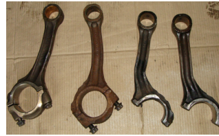
Broken Con-rod bolts
