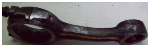
Bent Connecting Rod
