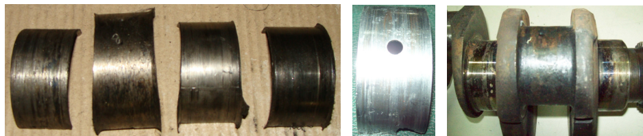
Badly worn Bearings Starvation of engine oil
