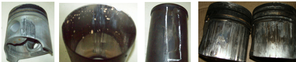
Severe scoring on Cylinder Liner & Pistons (Subjected to severe overheating due to defective Cooling system)
