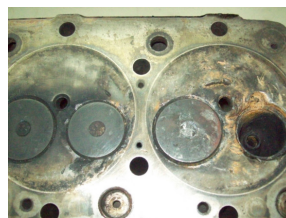
Valve Failure (Improper Tappet Setting)
