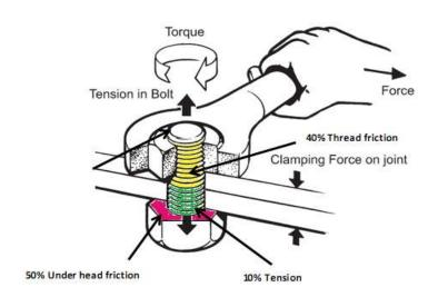
3.00 In conventional torque tightening, final torque values that are in Foot-pounds (Lb-ft) Or Newton-meter (N-m) alone is usually provided. This does not take into account the torque Lost in friction.
